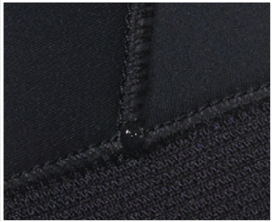
EXTERNAL SEAM REINFORCEMENTS
